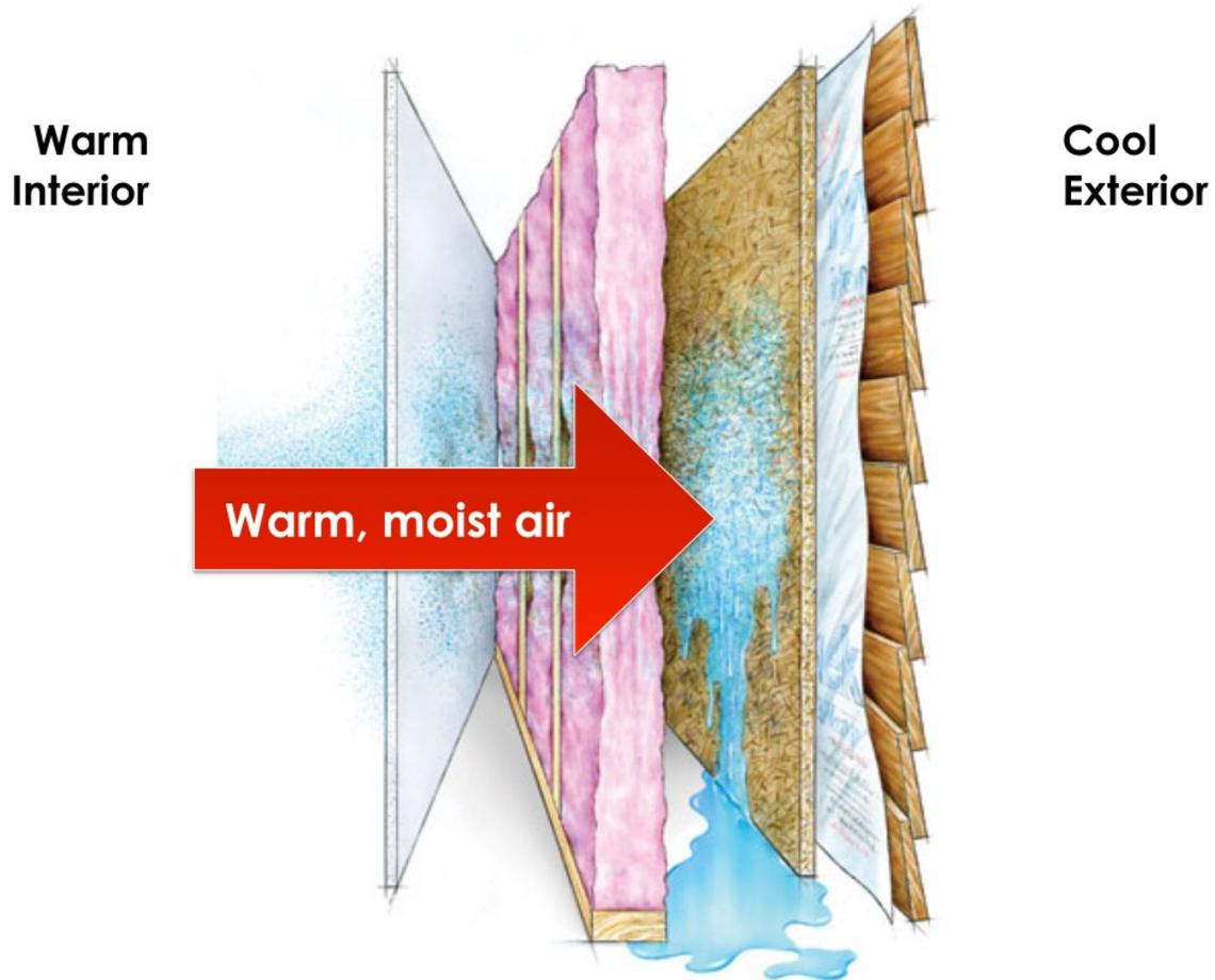
*Illustration showing the flow of moist air from the warm interior towards the cool exterior, condensing on the surface of the vapor retarder, courtesy Fine Homebuilding Magazine*
